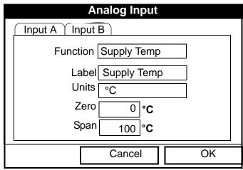
Figure 28: Analog Inputs Option Window - Energy Option Activated
